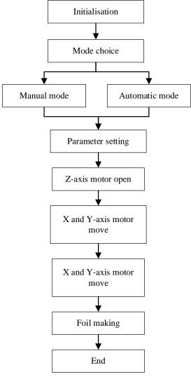
Figure 6: Control operation flow chart.
