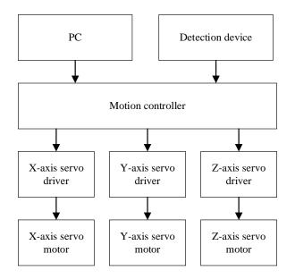
Figure 5: The system control principle.
